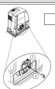
**NB!** The gearbox can be left in manual mode with the manual override hatch closed and locked up.
